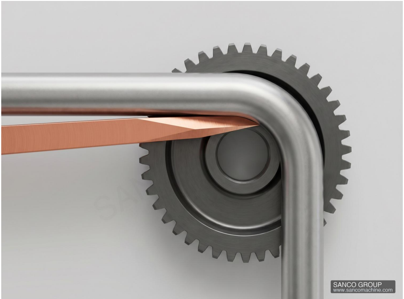
Figure 4 Schematic Diagram of the Position of the Copper Wiper Die in the Rotary Draw Bending Device — © SANCO GROUP · www.sancomachine.com
